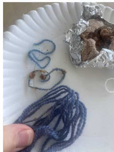
Photo: (Top two yarn samples) Kala Ilan after baking in a Barley Sourdough Starter, the top one is cleaned from baked dough. (Bottom yarn) Kala Ilan, Madder overdyed on Indigo, control for comparison.
